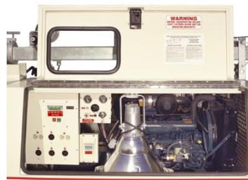
Light stowage inside the canopy comes standard to prevent damage during transportation or vandalism while the unit is unattended.
