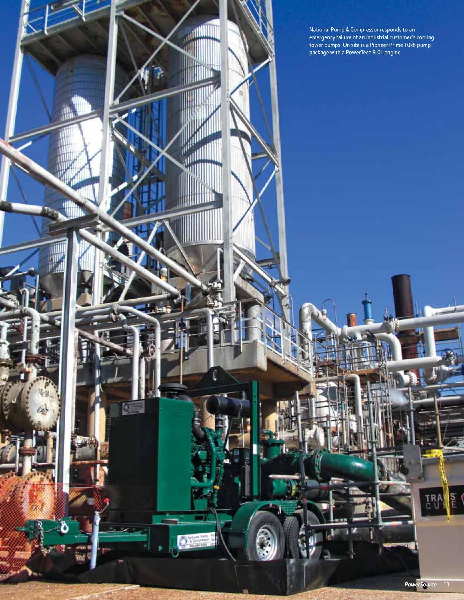
National Pump & Compressor responds to an emergency failure of an industrial customer's cooling tower pumps. On site is a Pioneer Prime 10x8 pump package with a PowerTech 9.0L engine.
