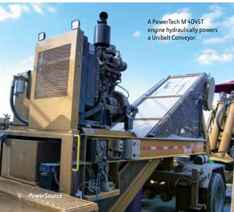
A PowerTech M 4045T engine hydraulically powers a Unibelt Conveyor.
