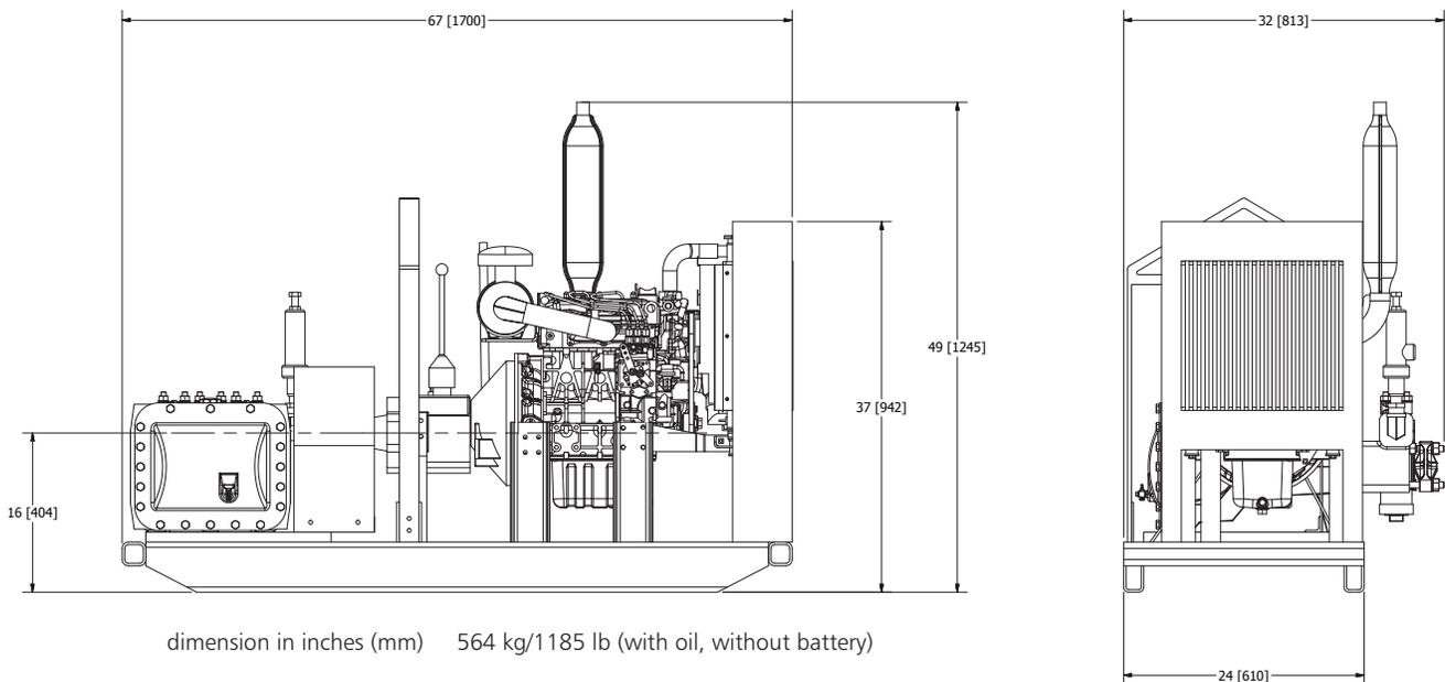
Diesel powered FMC (Bean) pumping unit designed for reliable service as a supply or pressure pump for core drilling. The diesel engine drives through a four speed transmission that is coupled to an FMC triplex piston pump. The pump can be operated with ball type valves for use with drilling mud or with disc type valves for use as a supply pump.
